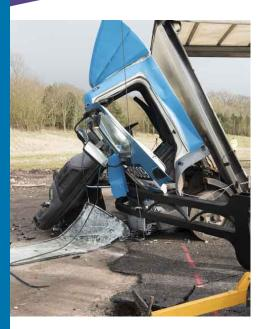
Eagle 'Fibre' technology Secure Before Impact (SBI) Tested on a 7.5T truck (N2A) at 64kph (40mph) Tested on a 1.5T car (M1) at 80kph (50mph) Very low penetration. Shallow foundation. Tested at 6m and 8m clear opening. Robust and rigid. Various designs available.
